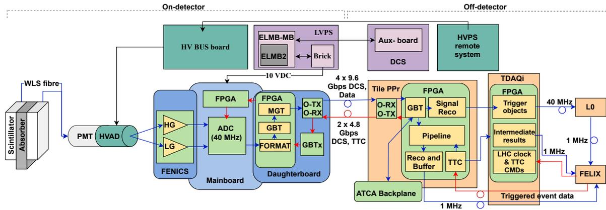
**Figure 1.** The HL-LHC Upgrade TileCal readout chain and power distribution system.
